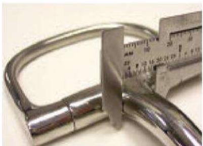
Diameter of bit is measured at the rings or cheeks of the mouthpiece.
